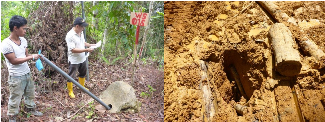
Figure 3.13 Drillhole azimuth and dip checks using PVC pipe inserted into the collars (LHS) and the WS-005 collar remains.
