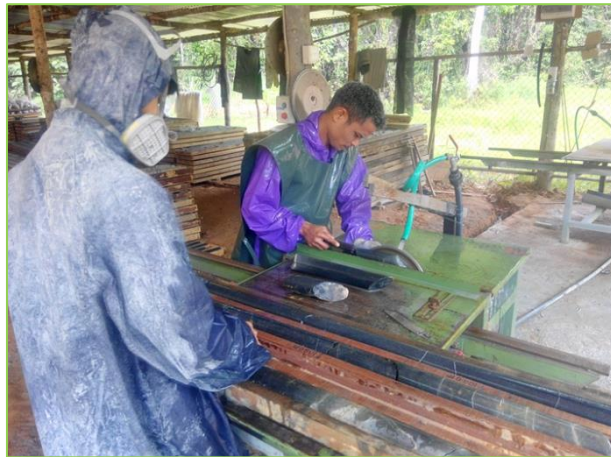
Figure 3.23 Core cutting using a diamond tipped saw
