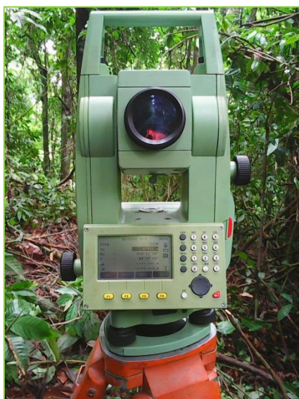
Figure 3.17 Survey total station unit and concrete collar with casing and hole details
