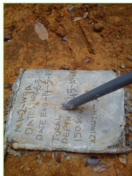
Figure 3.17 Survey total station unit and concrete collar with casing and hole details
