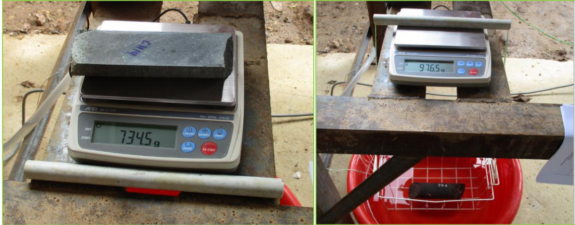
Figure 3.26 Density measurement scales showing dry weight (left) and weight in water (right)
