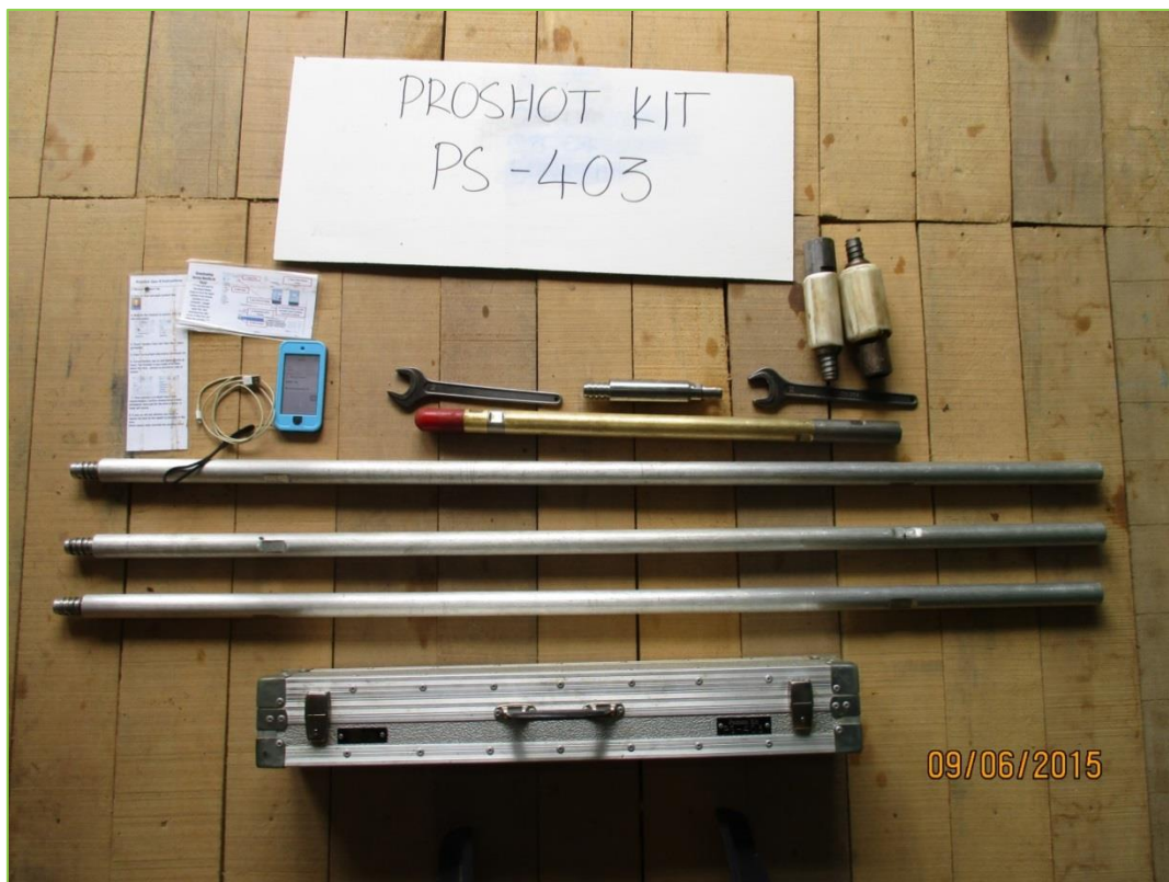
Figure 3.20 Camteq Proshot PS-403 EMS survey tool and accessories
