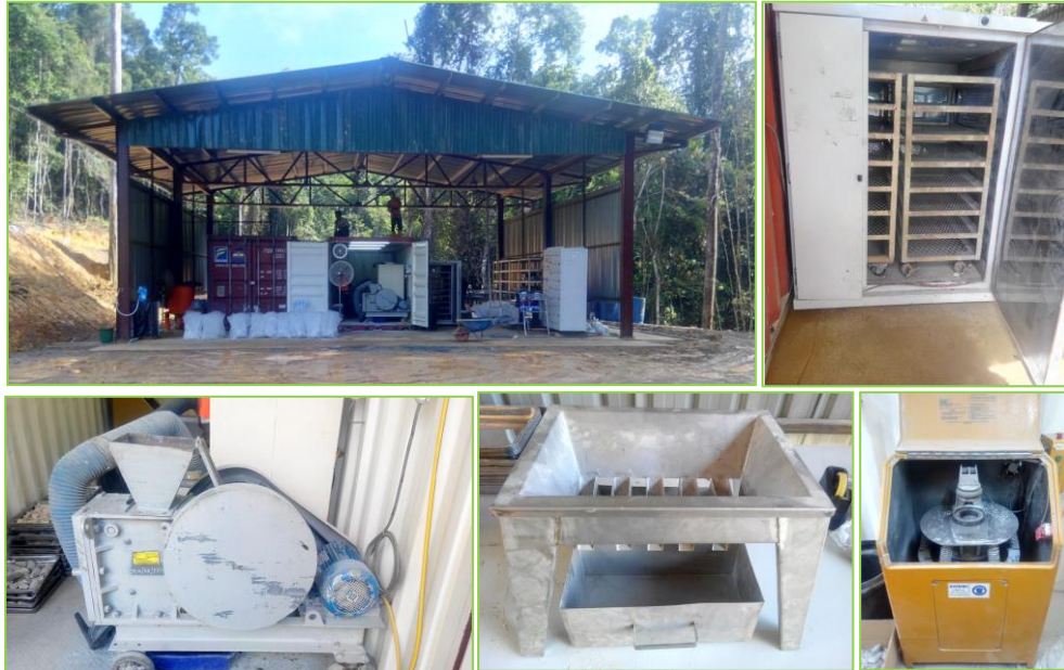
Figure 3.24 SGS Mineral Services Mobile Sample Preparation Unit (MSPU)
